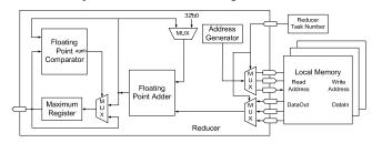
Figure 9. The internal structure of reducer
