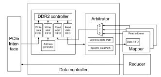
Figure 10. The internal structure of data controller
