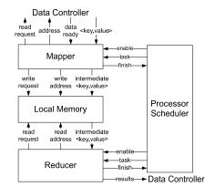
Figure 4. The data exchange between mappers and reducers
