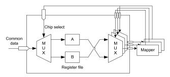
Figure 6. The internal structure of common data path
