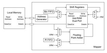
Figure 8. The internal structure of mapper
